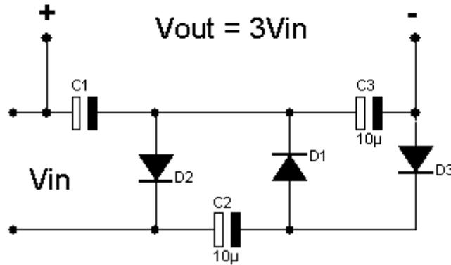
Figure A.1-2: Voltage Tripler
