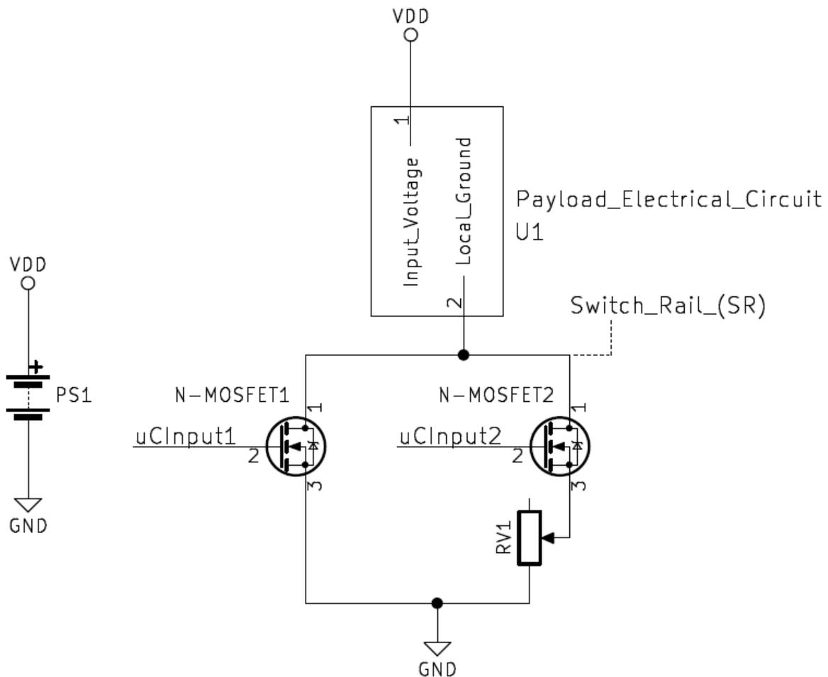
Figure A.2-1: Electronic Voltage Switch Circuit
