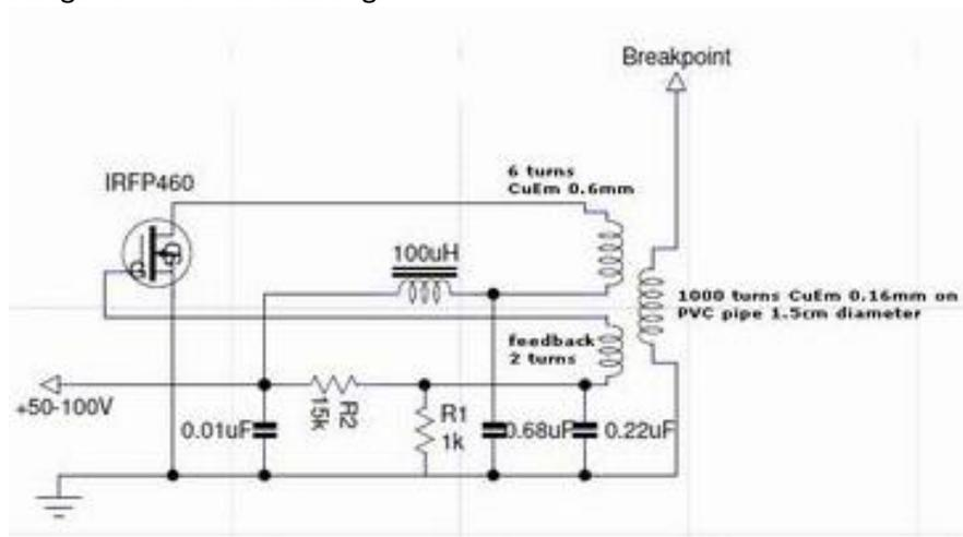
Figure A.1-1: High-Frequency Tesla Coil Design
